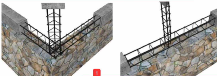
Figure 3: The Triadic Colomn to Reduce the Building Structure Material
