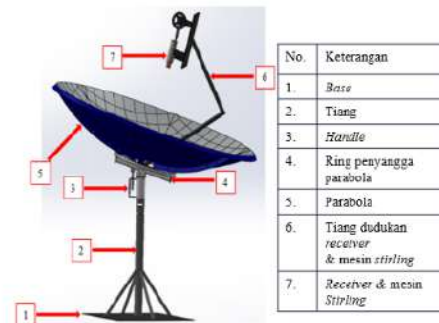
Gambar 1. Skema peralatan CSP (Priagung, 2019)
