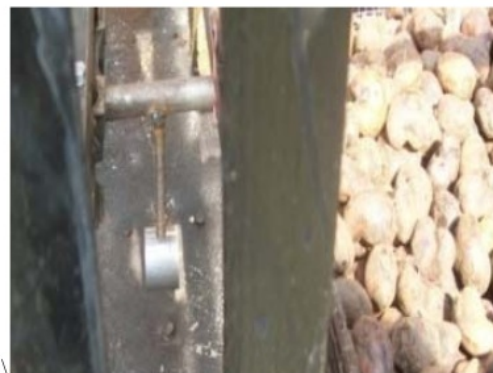
Figure-3. An unbalance mass is placed under the shelves.
