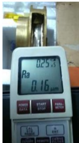
Figure 3. Surface roughness measurement
