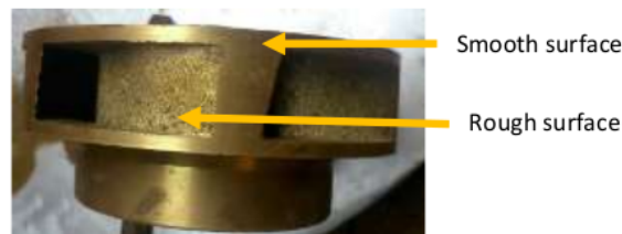
Figure 1. The surface condition of the original impeller
