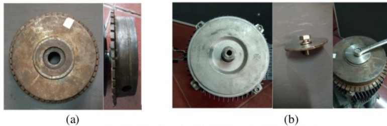
Figure 7. (a) The flywheel, (b) Flywheel installation.
