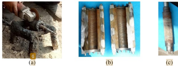
Figure 5. Modification of rotor (a) cage cutting, (b) cut cage, (c) shaft.
