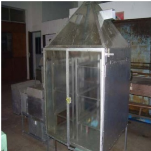
Figure-1. Green dryer machine by using vibration components to dry RDF and/or agricultural products.
