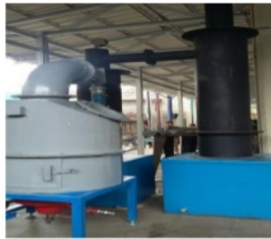
Figure 10: RDF Burning Chamber, Cyclone and Wet Scrubber.
