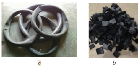
Fig. 1. Scrap tires: a – bulk tube-type tire; b – pieces of scrap tire
