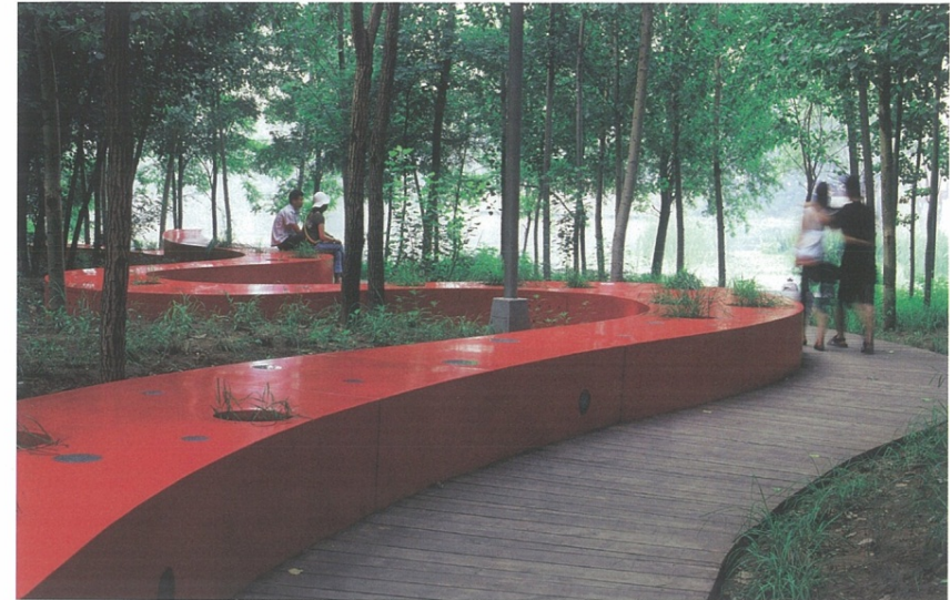
The "red ribbon" is made of steel fiber and lit from its interior so that it glows red at night. It stands 2-inches-tall and 1-5 in in width. Various plants grow in strategically placed holes in the ribbon.
